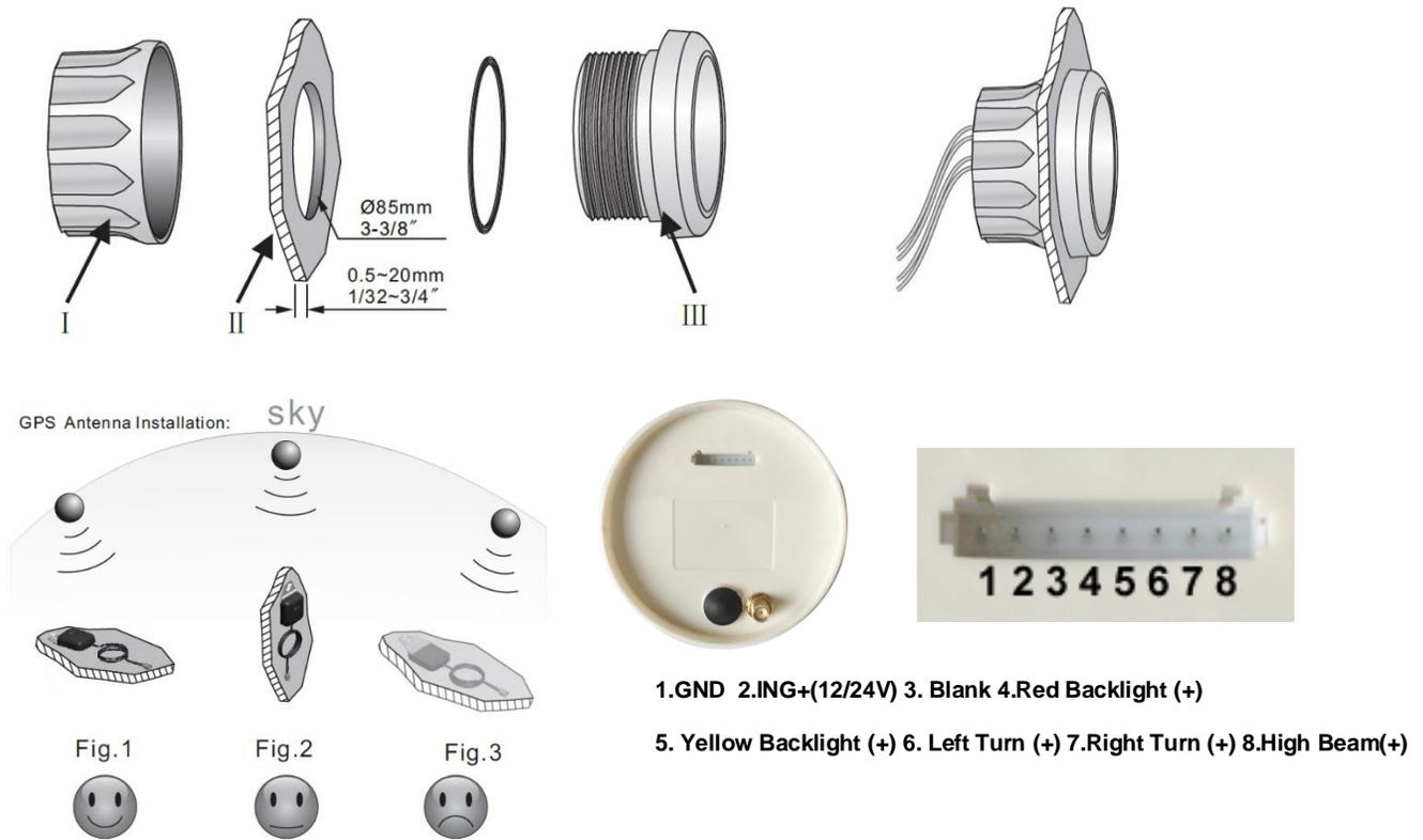
1. Cut an 85mm (3 3/8") hole in the panel (II) and allow a clearance of 55mm (2 3/16") behind the panel to fit the gauge.
