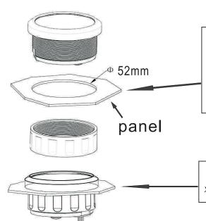
Before installation, firstly, to open a hole  $\Phi$ 52mm of the panel ,make sure there is a space with (55mm backyard of panel)as well.
