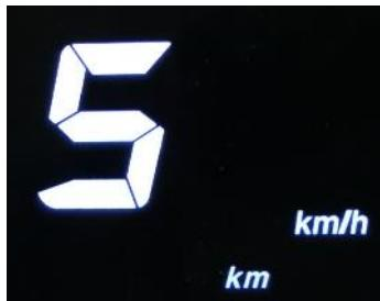
The 188 second 8-character display of the speed display shows 5, the lower right corner displays km / h, short press km / h (metric) and mph (imperial) to switch.
