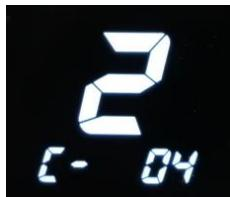
188 second 8-character display with speed display 2 and total accumulative display C-04, 04 indicates the number of magnetic steel, 1-12 can be set
