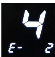
The 188 second-digit 8-character display of the speed display shows 4, the total cumulative display is E-2, 2 indicates a two-line (8 / 98 Ω ) oil gauge, and 3 indicates a three-line (33 / 566 Ω ) oil gauge
