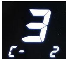
The 188 second-digit 8-character display of the speed display shows 3, and the total cumulative display shows C-2.
