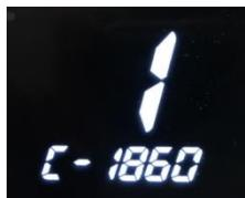
The 188 second 8-character display of the speed display shows 1, the total cumulative display is C-1860, 1860 means the default tire circumference is 1860mm, thousands of flashes, short press the left button to start changing the current digits, and no movements will flash the hundreds. Cycle to the singles.
