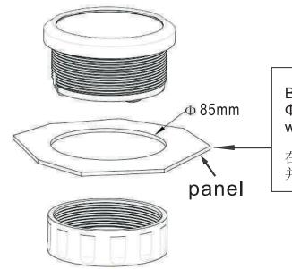
Before installation, firstly, to open a hole Φ85mm of the panel ,make sure there is a space with (55mm backyard of panel) as well.
