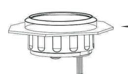
Put the gauge in the hole and screw down.
