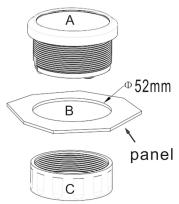
Picture B: Before installation, firstly, to open a hole Φ52mm(2-1/16") of the panel, make sure there is a space with (55mm backyard of panel) as well.
