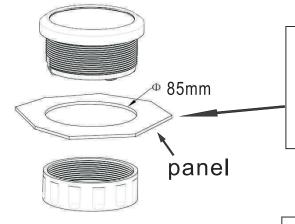
Before installation, firstly, to open a hole Ф85mm of the panel ,make sure there is a space with (55mm backyard of panel) as well.
